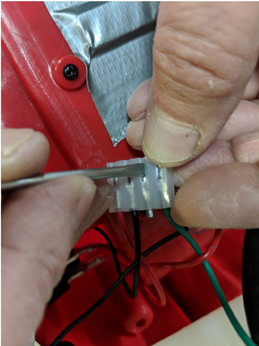
Figure 3: Push in using the screwdriver to release the connector, it can then be taken out from the bottom of the wiring harness.
