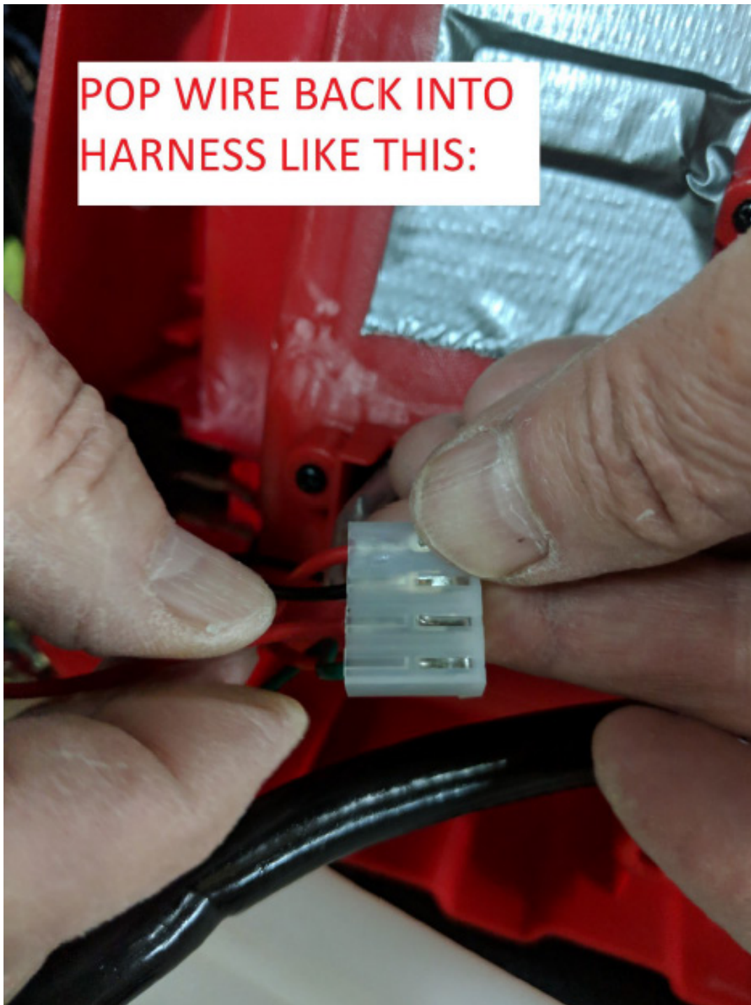
Figure 10: Once back in place, the small tab will click. Once in place, it should not be able to pull back out.
