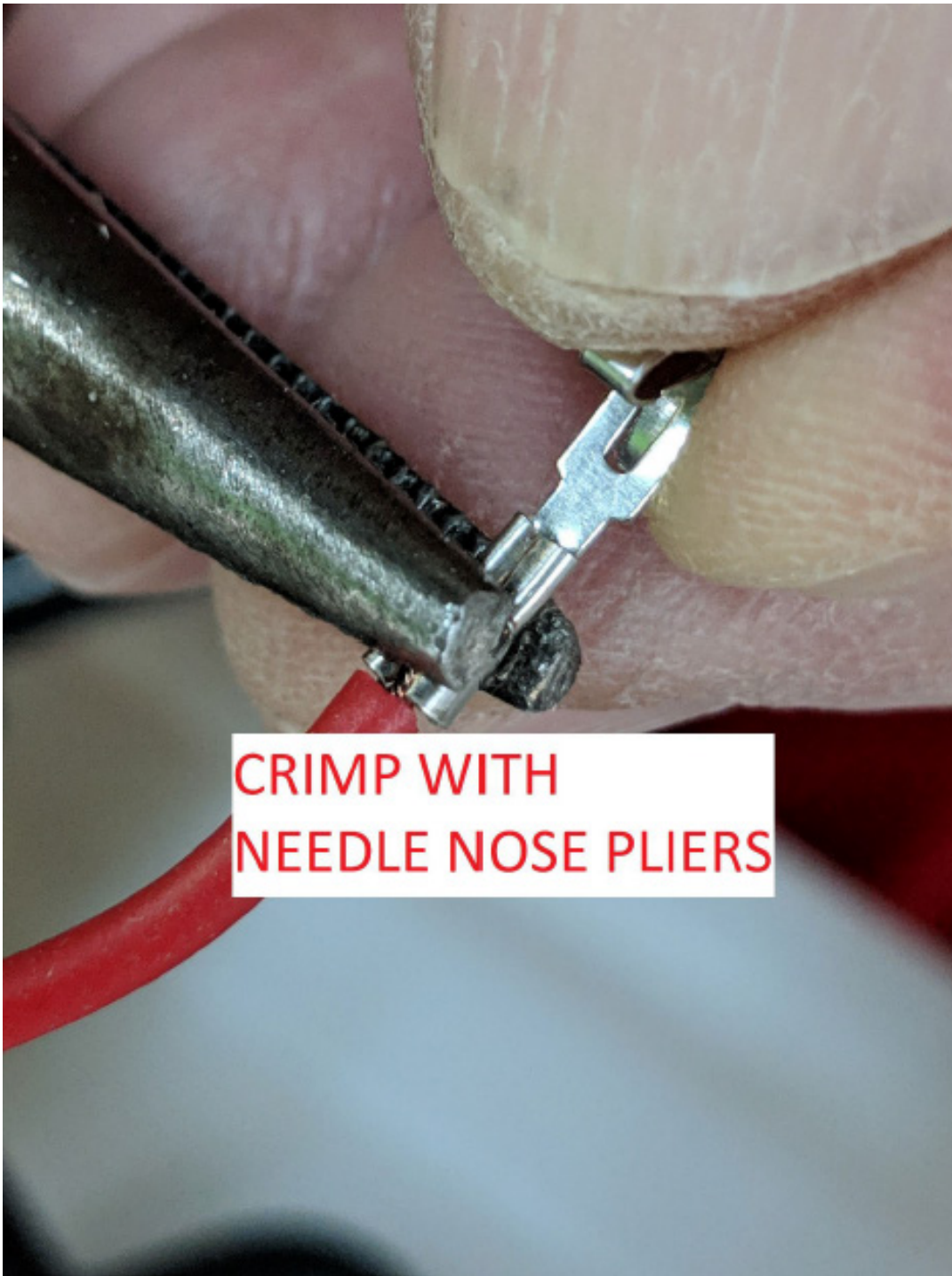
Figure 7: Crimp down on the connection to hold the copper wire against the silver connector.
